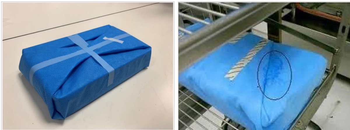
Figure 1: a) The [REDACTED] blue wrap 11 and b) rapid cooling can lead to droplet condensation, dripping and localised wet spots, which may allow bacteria to wick through the porous barrier and compromise the sterility of its contents. 14
